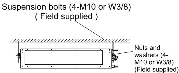
Fig. 3.4 The installation of the indoor unit
